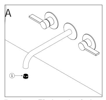
Unscrew the aerator (1) from the spout, then, pull out the aerator and soak it in a vinegar and water solution to remove lime build-up. Once parts have been cleaned, reassemble by reversing steps.
