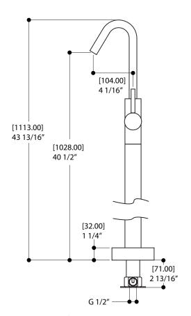
Flow rate: 2.2 gpm
